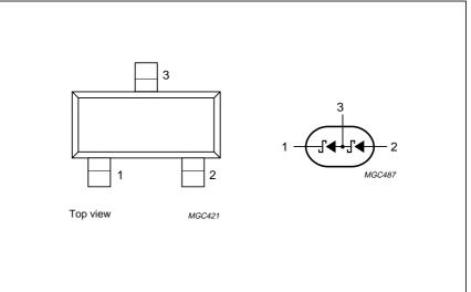
Fig.1 Simplified outline (SOT23) pin configuration and symbol.
